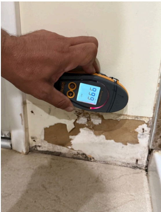
Side of the stand-up shower showed high moisture readings and visible contamination along the lower portion of the wall.
